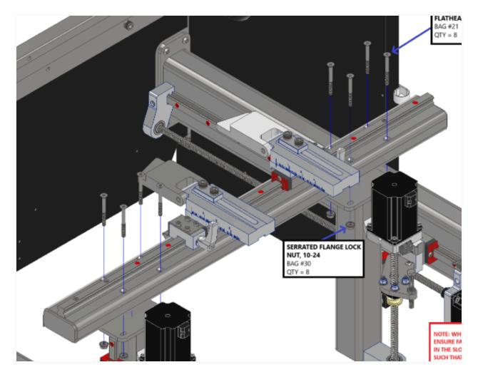
3. Run the unit up and down and look at the behavior of each R-axis assembly when they are not connected to each other.
