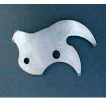
The type and size of lead-in and lead-out can significantly affect cut quality, particularly with bolt-holes and slots. Two common defects are divots and bumps. A divot occurs when the arc removes too much material at the end of the cut. As the plasma arc crosses the lead-in kerf – the removed material from the beginning of the cut – it transfers to the saved part, causing a small indentation or, sometimes, a larger scooped-out region. This makes the hole out-of-round.
