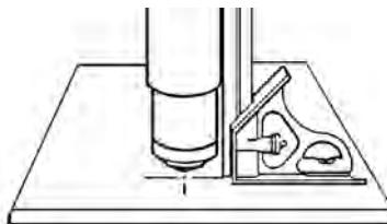
Note: Check to see if material is bent or warped; in extreme cases this limitation cannot be corrected.
