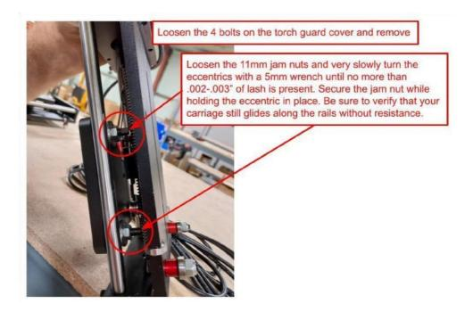
Check for binding along the vertical guide rails. The slide should move smoothly when jogged in both Z-directions. There should be no binding or sudden drop, caused by the slide failing to move in unison with the lead nut. If you witness this, adjust the V-rollers along the right side of the Z-slide.
