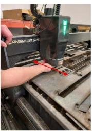
Check at each end of the gantry tube as well as the center and tighten the bearings set while tramming as needed. If there is solid contact between the bearings and the gantry tube and lash is still present, remove the torch guard cover and adjust the V-rollers along the right side of the Z-slide.
