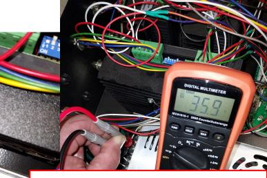
Continue adjusting the voltage until you are as close to 36V as possible.
