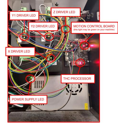
Check your voltage by probing any pair of the smaller black and white wires with a digital multimeter. The nominal DC voltage setting is 36V so any other measurement will require adjustment.
