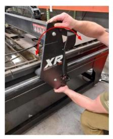
Check each side at the front, center, and rear of the Y - axis rails and adjust the lower V-roller as necessary so that it is in constant contact with the rails. Do not overtighten, simply adjust until the roller contacts the rail. Lastly, check for lash in the X/Z carriage by gently grasping the torch body and rocking along the Y axis.
