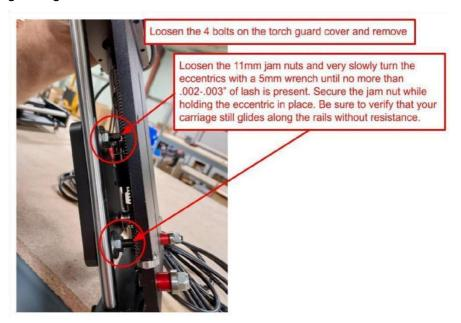
Do not overtighten. Gently lift the torch in the slide with your finger and let it drop. The torch and slide must lower along the rails under their own weight, thus ensuring the IHS switch remains in constant contact with the lead nut as it travels downward. If it sticks or drops, adjust the V-rollers as needed.
