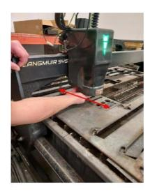
Check at each end of the gantry tube as well as the center and tighten the bearings set while tramming as needed. If there is solid contact between the bearings and the gantry tube and lash is still present, remove the torch guard cover and adjust the V-rollers along the right side of the Z-slide.
