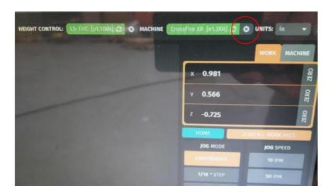
Disconnecting from FireControl before powering down the table will prevent the MC4000 computer from rebooting.
