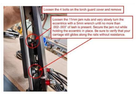
Check for binding along the vertical guide rails. The slide should move smoothly when jogged in both Z-directions. There should be no binding or sudden drop, caused by the slide failing to move in unison with the lead nut. If you witness this, adjust the V-rollers along the right side of the Z-slide.
