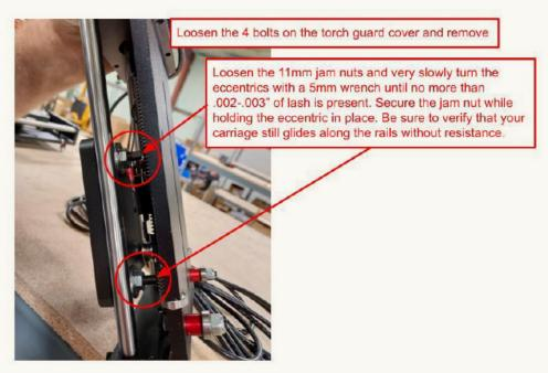
Do not overtighten. Gently lift the torch in the slide and be sure that the slide will still lower along the rails under its own weight.
