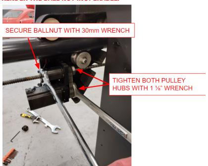
Hold the ball nut in place with a 30mm wrench and secure the pulley hubs by tightening the 2 nuts with a 1 1/8" wrench. Be careful not to damage the polymer pulley with excessive force. Replace the rear rail mount assembly. Do not apply excessive force when tightening the cinch bolt against the rail. It needs only to be snugged in order to secure it. Overtightening can cause misalignment.
