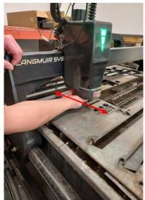
Check at each end of the gantry tube as well as the center and tighten the bearings set while tramming as needed. If there is solid contact between the bearings and the gantry tube and lash is still present, remove the torch guard cover and adjust the V-rollers along the right side of the Z-slide.
