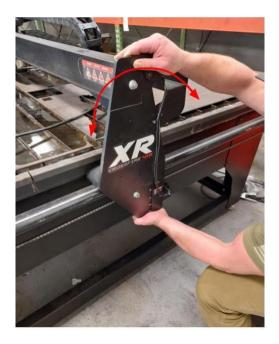
Check each side at the front, center and rear of the Y - axis rails and adjust the lower V-roller as necessary so that it is in constant contact with the rails. Do not overtighten, simply adjust until the roller makes contact with the rail. Lastly, check for lash in the X/Z carriage by gently grasping the torch body and rocking along the Y axis.
