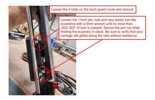
Do not overtighten. Gently lift the torch in the slide and be sure that the slide will still lower along the rails under its own weight.
