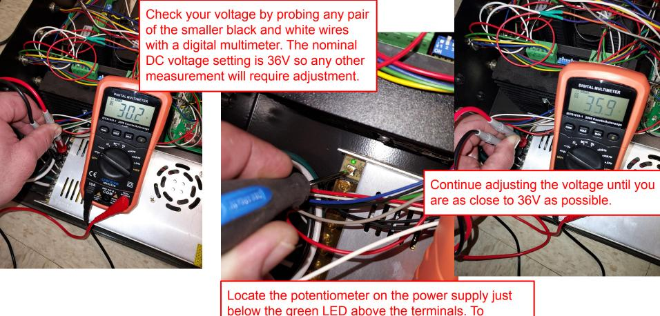
Locate the potentiometer on the power supply just below the green LED above the terminals. To increase the voltage slowly turn the pot clockwise. A few degrees either direction is enough to adjust several volts so adjust CAREFULLY.
