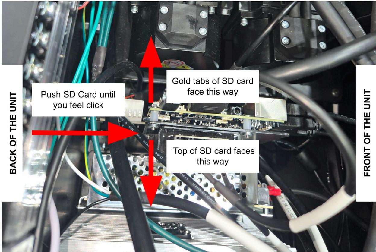
3. Install the updated micro SD card. If you are facing the back of the unit, the golden tabs of the micro SD card must face towards your left. The card must be locked into place. You will feel/hear a discernible click when the card is locked in.
